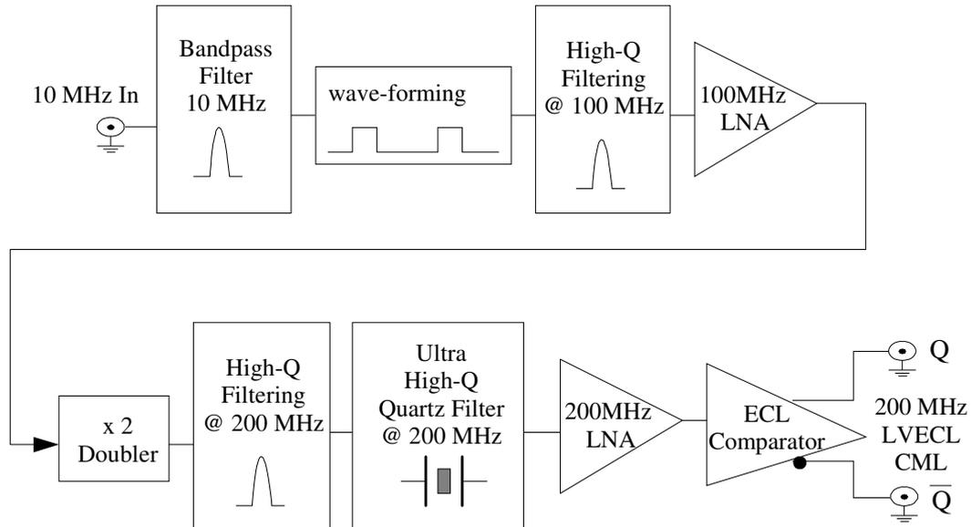
Fig. 2: Block Diagram of 200 MHz Frequency Multiplier
