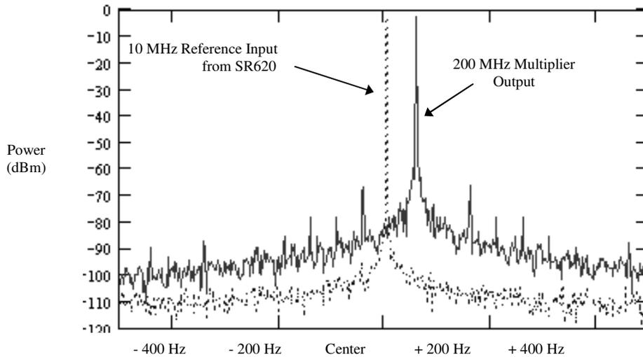
Fig. 6: Carrier Deterioration due to Frequency Multiplication Process
